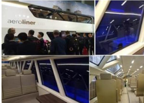
*Full-scale mockup of the AeroLiner3000, with Vision Systems Nuance brand of SPD-Smart EDWs (Electronically Dimmable Windows) – shown in a darkly tinted state at top right and bottom left.*
