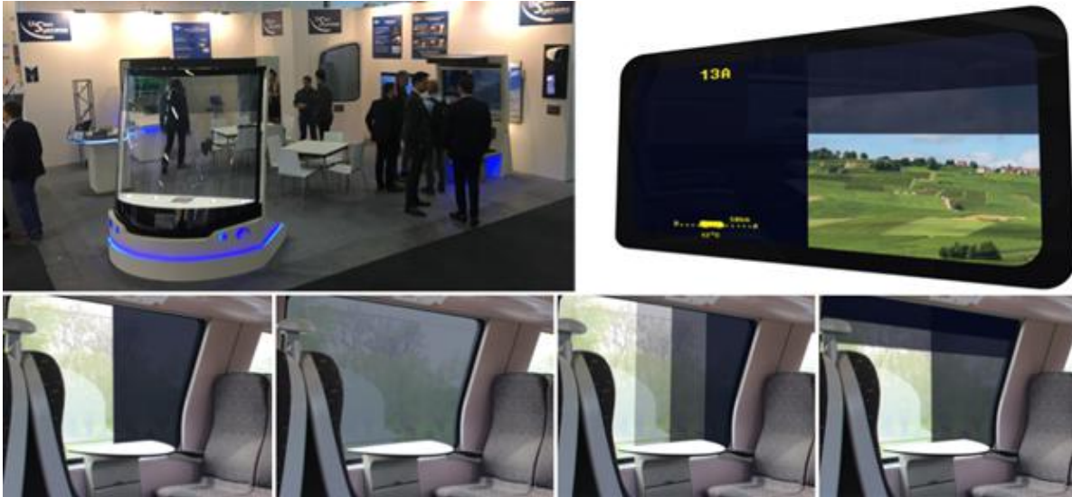
At top: Vision Systems booth at 2018 InnoTrans, and Info-Vision window integrating an electroluminescent display into an SPD-SmartGlass electronically dimmable window (EDW). At bottom: Vision Systems Nuance V2 Multizone SPD-SmartGlass EDW, with various zones being controlled for maximum comfort.
