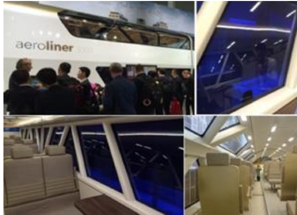
Full-scale mockup of the AeroLiner3000, with Vision Systems Nuance brand of SPD-Smart EDWs (Electronically Dimmable Windows) – shown in a darkly tinted state at top right and bottom left.
